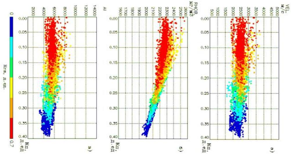
Figure 1 – Dependences of Vp, AI, DENSITY on porosity with color-coded clay.
