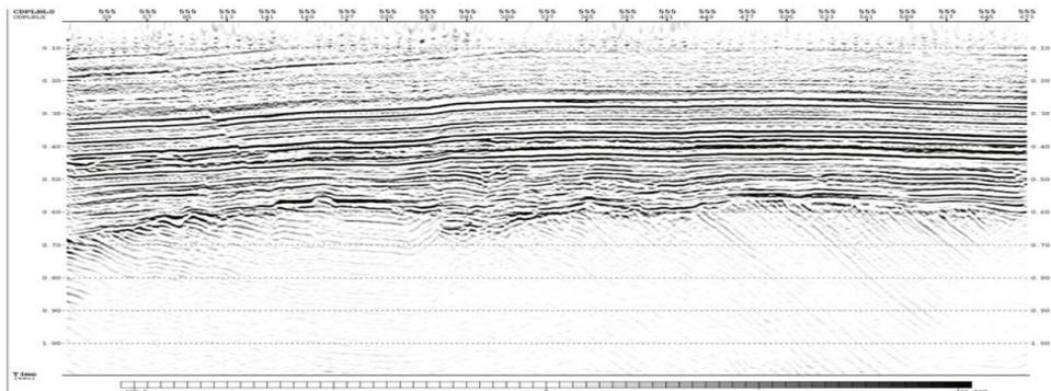
Figure 5 – Final total depth section recalculated to the time scale
