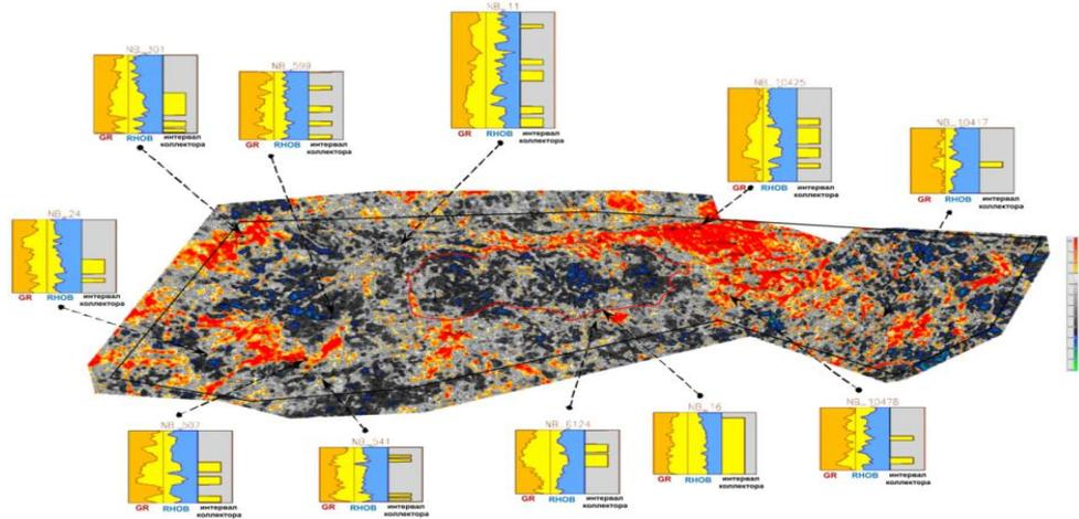
Figure 2 – Fluid Factor attribute amplitude distribution for reservoir B
