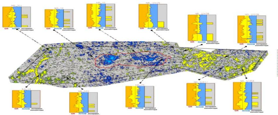
Figure 3 – The distribution of the amplitude of the attribute  $\Lambda * \text{Rho}$  Reflectivity in the reservoir G2
