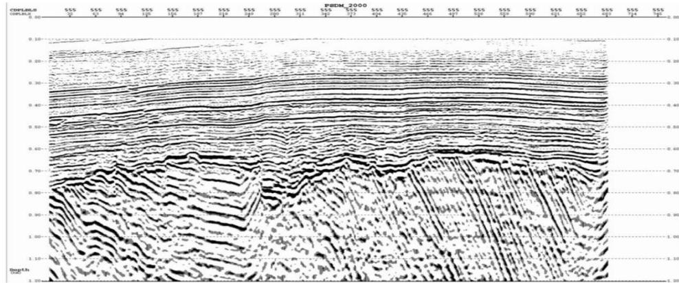
Figure 1 – Total section PSDM aperture 2000 m.
