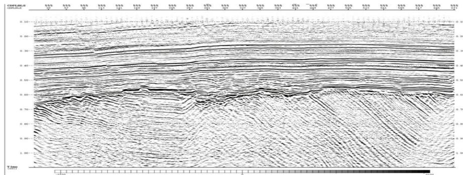
Figure 6 – The final total depth section, recalculated to the time scale with processing after summation. Line 555
