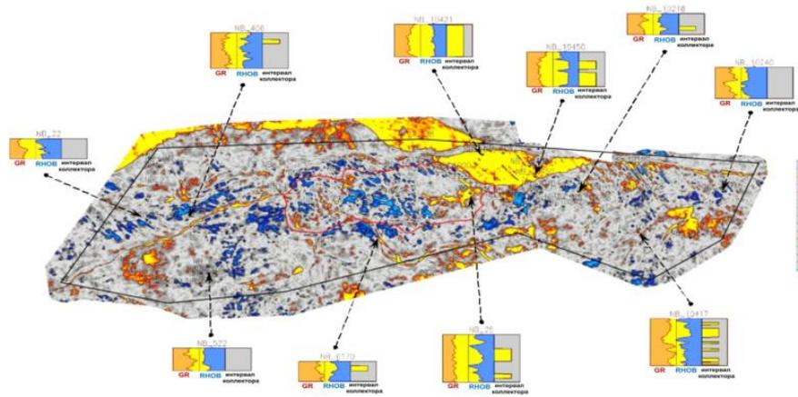
Figure 1 – Distribution of the amplitude of the Normal Incidence Reflectivity (R0) attribute over for Reservoir A2
